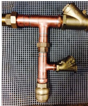
Figure 2: Recirculation Manifold (‘R’)
